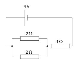
What power is dissipated in one of the  $2\Omega$  resistors and in the whole circuit?
