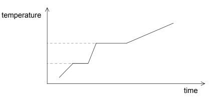
The specific heat capacities of the solid, liquid and gaseous forms of the material are  $c_s$   $c_l$  and  $c_q$  respectively. What can be deduced about the values of  $c_s$   $c_l$  and  $c_q$ ?
